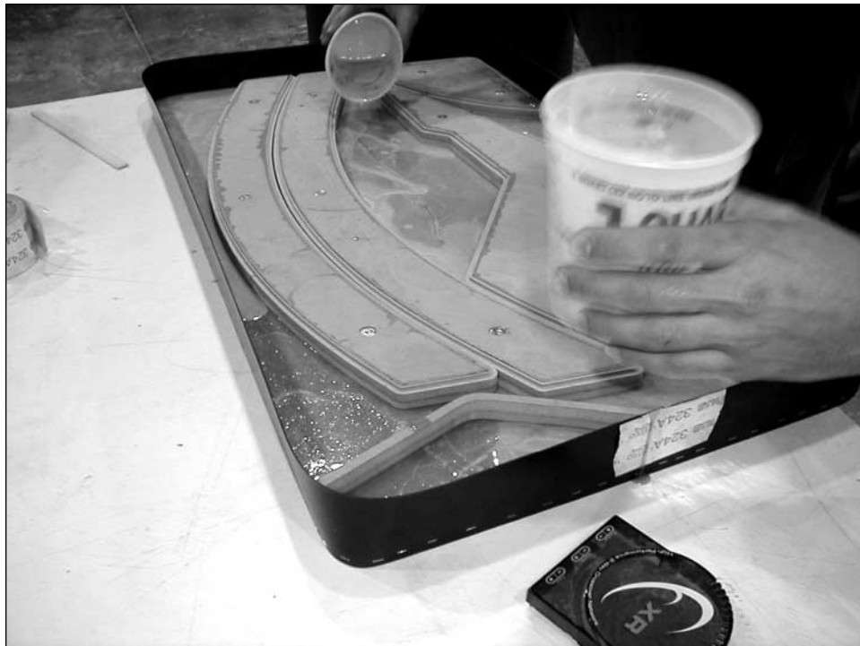
Two-part expanding foam is poured onto the panel.
