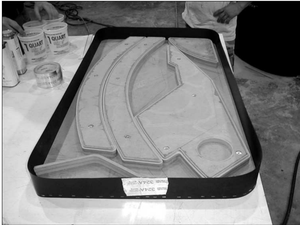
An ABS Plastic frame is stapled to the perimeter of the door base to create a barrier.
