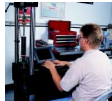
Testing a Koni 3012 on a computerized shock dyno.
