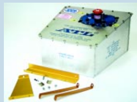
170120 Porsche 911 - 17 Gallon Cell - Accepts OEM Porsche Fuel Sending Unit
